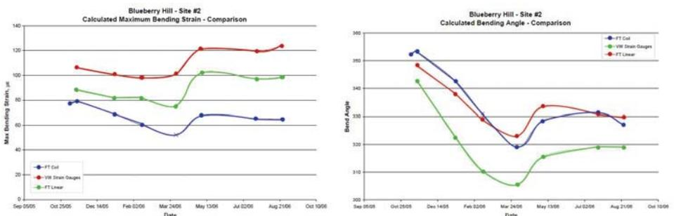
**Figure 6:** (Left) Maximum bending strain, and (right) bending angle of pipeline at Site #2, located ~100 meters uphill from the Blueberry River.
