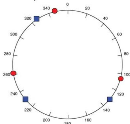
**Figure 5:** Angular location of FT Linear Sensors (blue squares), and FT Coil Sensors (red circles). Product flow was to the south.
