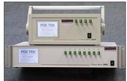
**Figure 3:** FT 3410 (top) and FT 3405 Monitor for FT Sensors
