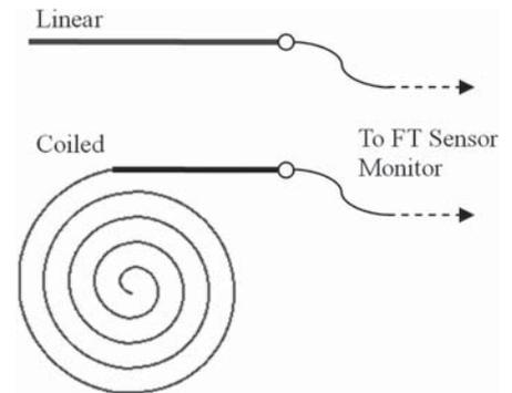
**Figure 2:** Linear and Coiled FT Sensors Sensor Monitoring
