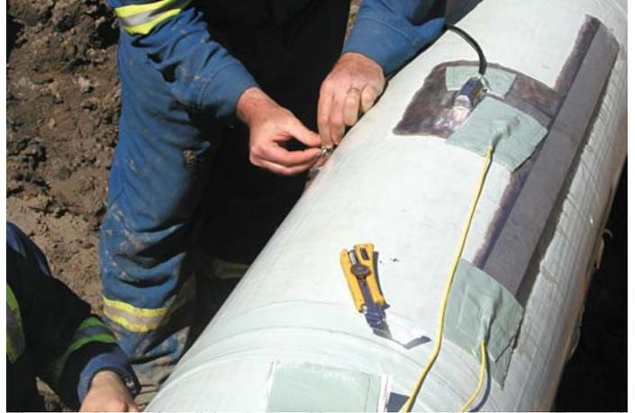
**Figure 4:** Photo of daylighted pipe with exposed, bonded sensors. From left to right, visible sensors are a VW strain gauge, 10 m coiled FT Sensor, and a 1 m linear FT sensor.
