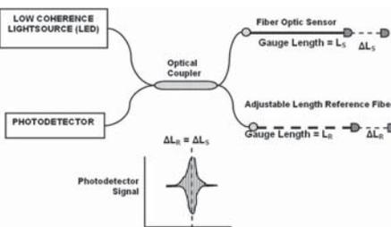
**Figure 1:** FT Fiber-Optic Sensor system schematic
