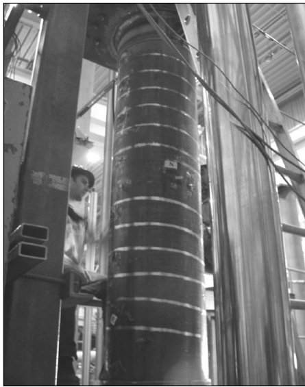
A compression machine at the University of Alberta tests a pipe spiral wrapped with an FT sensor for failure due to internal pressure, axial compression, and bending loads (Fig. 2).
