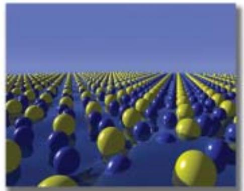
This image represents periodically ordered gold (yellow) and silicon (blue) atoms within the surface-frozen monolayer of liquid gold-silicon eutectic alloy. Courtesy of BNL.
