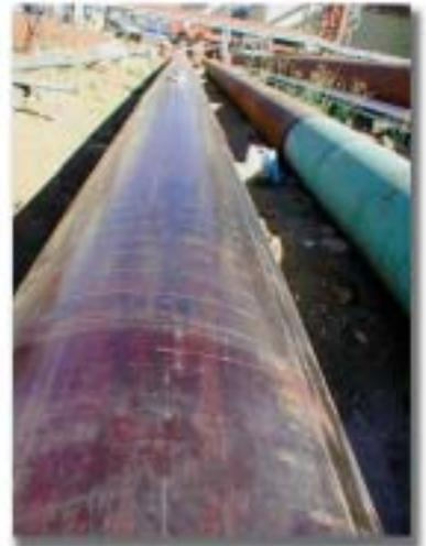
Here, a fiber optic sensor is bonded to a tailings pipe in a serpentine configuration. Courtesy of FOX-TEK.
