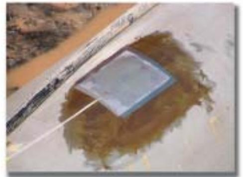
A close-up view of a fiber optic sensor designed to monitor local wall thinning, a technology patented by a Toronto-based, fiber optic technology company. Courtesy of FOX-TEK.
